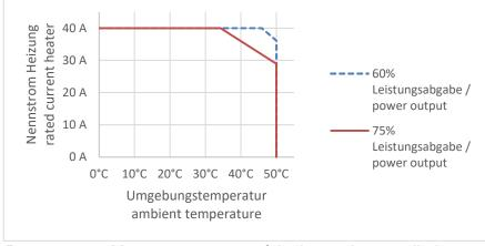
Power output: Mean power output of the heater in controlled state
